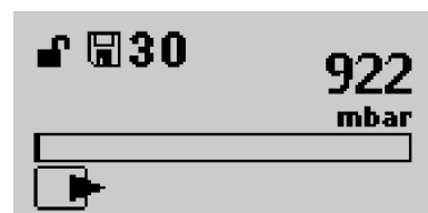
Fig. 32: Evacuation status display (047)
