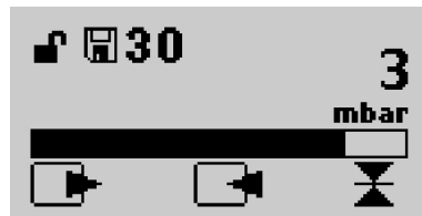
Fig. 34: Sealing status display (050)
